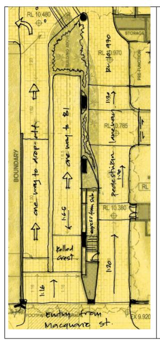
Revised planter and column cladding zones along the vehicle entry ramps to increase the width of the north-south link and improve the pedestrian throughfare width along these shopfronts (with ability to introduce seating elements if desirable by landscape architect)
